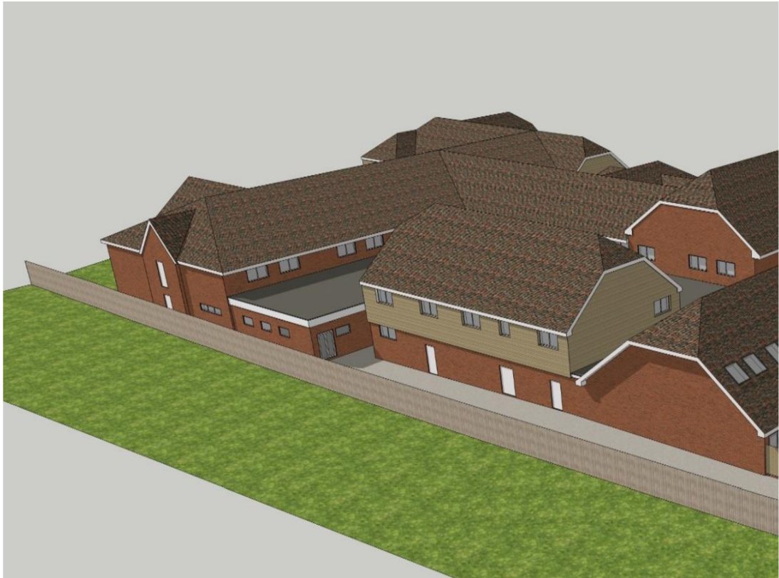
Figure 1 – 3D model of southern elevation of existing hotel identifying flat roof structure to be removed as part of proposed works
