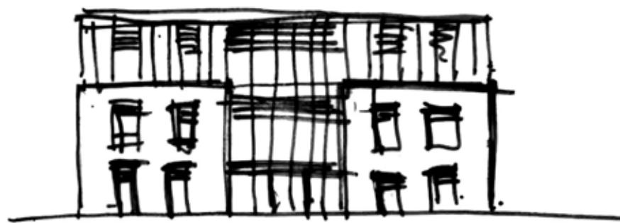
7. The sketch adds a lighter-weight top floor to reduce the building's overall weight; and also be sympathetic to the design of both the adjacent existing office and the facing residential units with have a sense of "base" and top"
