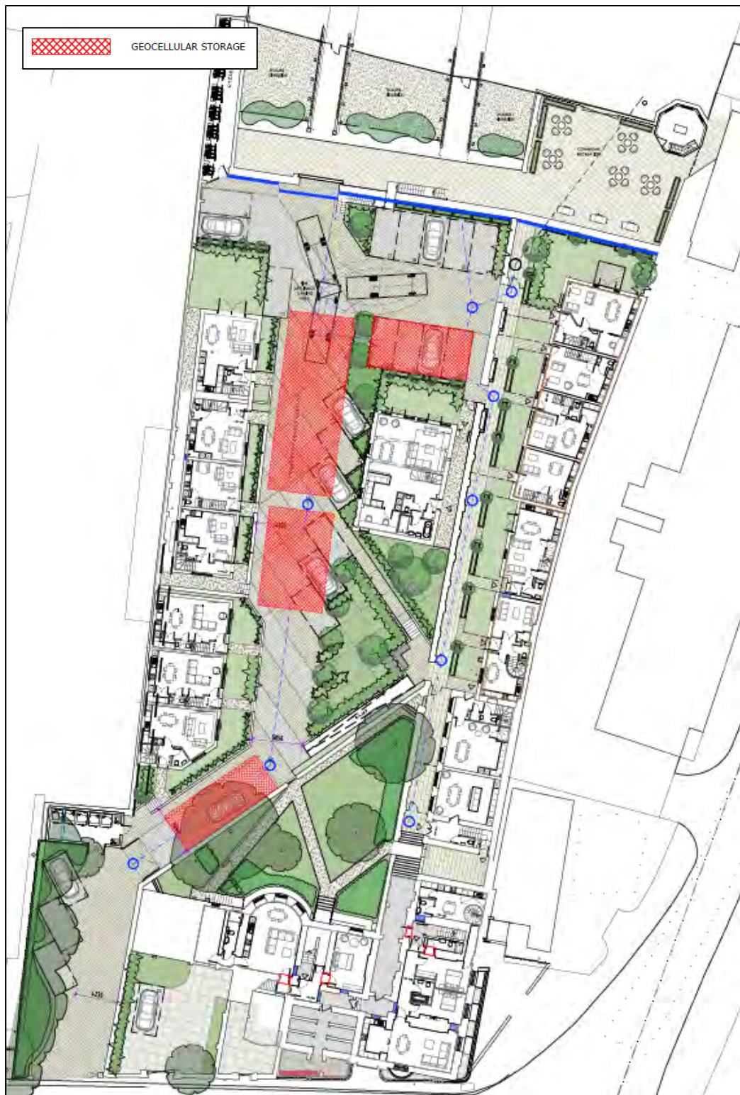
Figure 8.1 - Indicative drainage layout plan showing the proposed location of SuDS.
