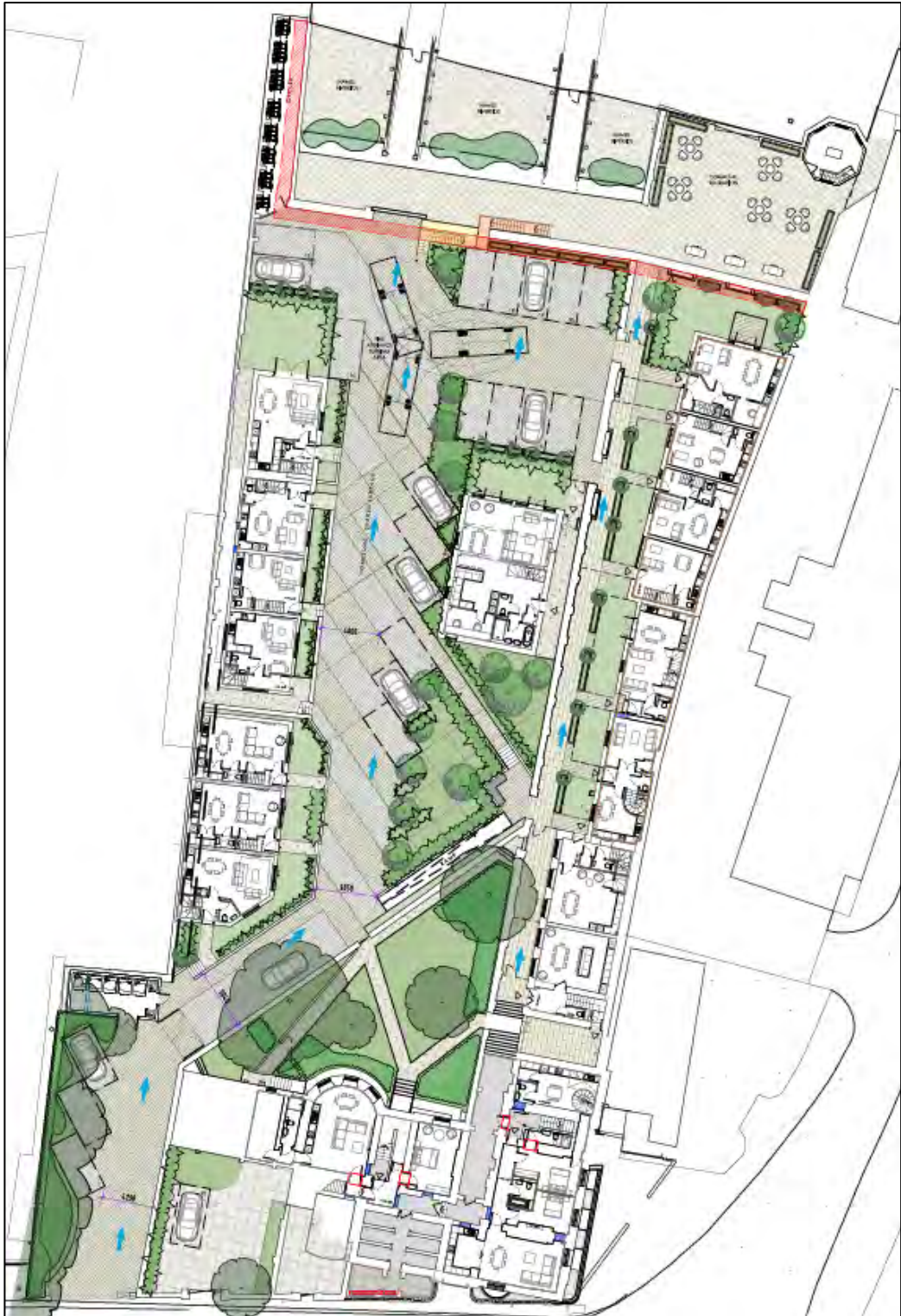
Figure 8.2 – Anticipated flow routes during an exceedance or blockage event.
