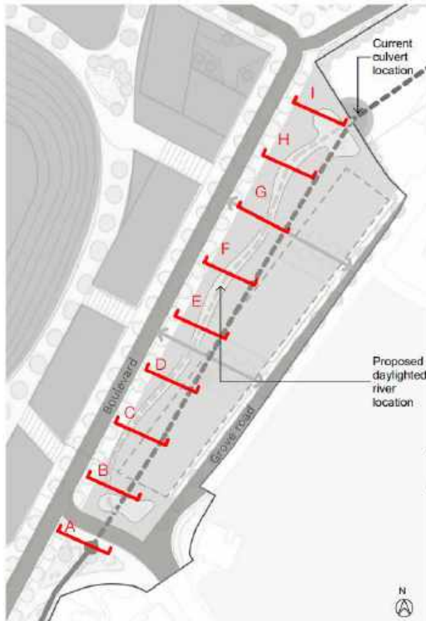
Figure 4-2: Daylighted channel section locations (HLM Architects)
