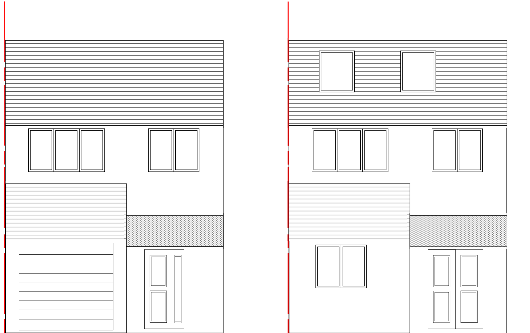
Existing Front Elevation
