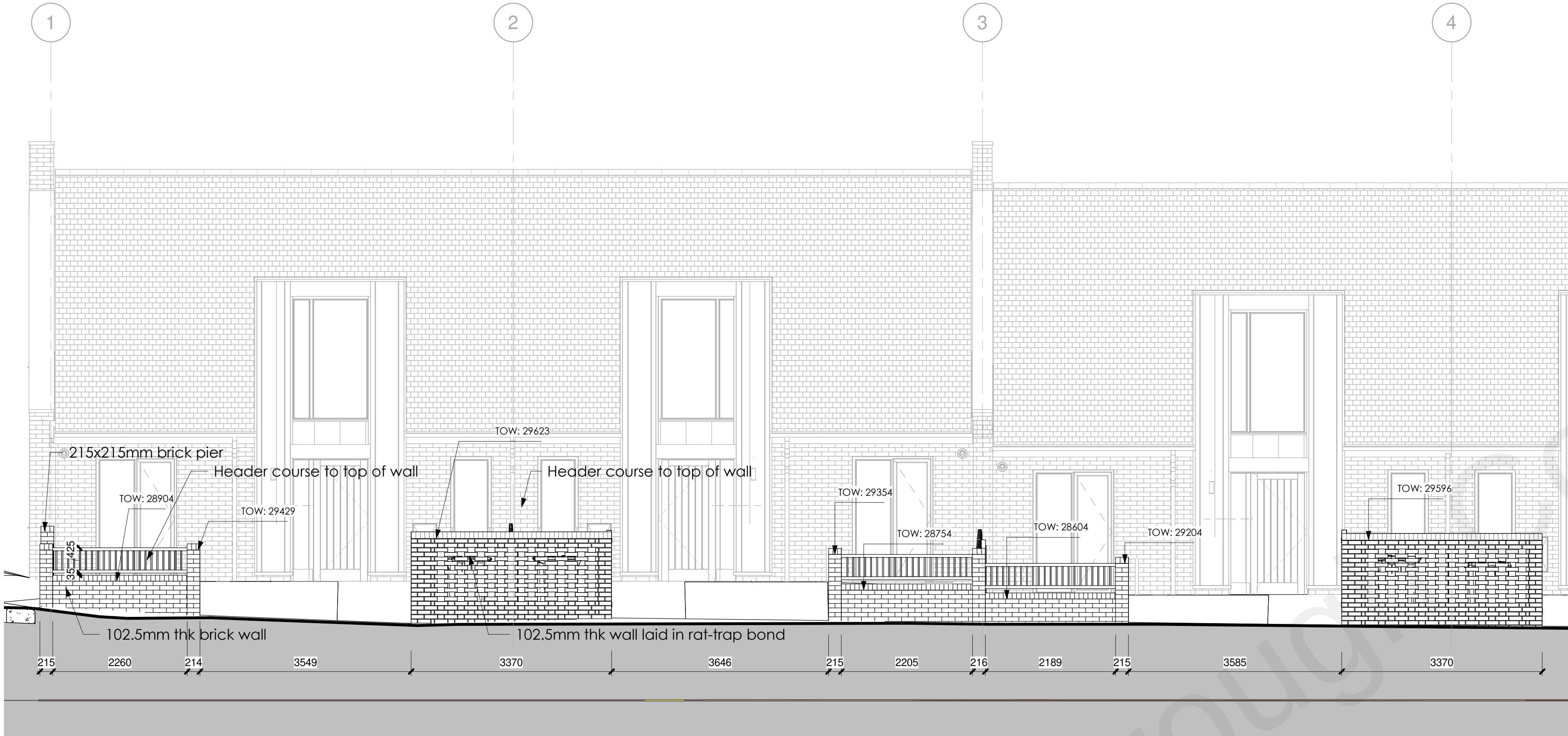
1 Garden Wall West Elevation Part 1 1 : 50
