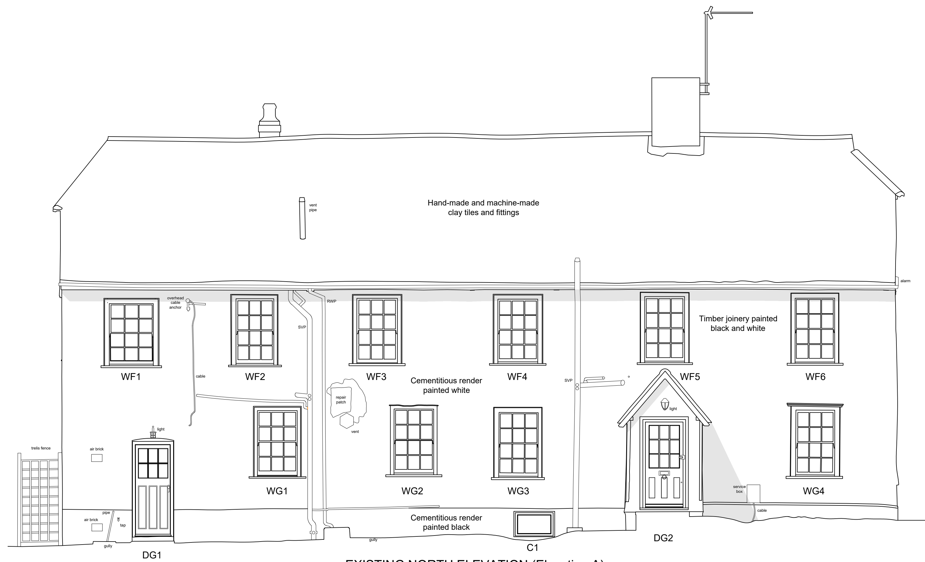
EXISTING NORTH ELEVATION (Elevation A) SCALE 1:50
