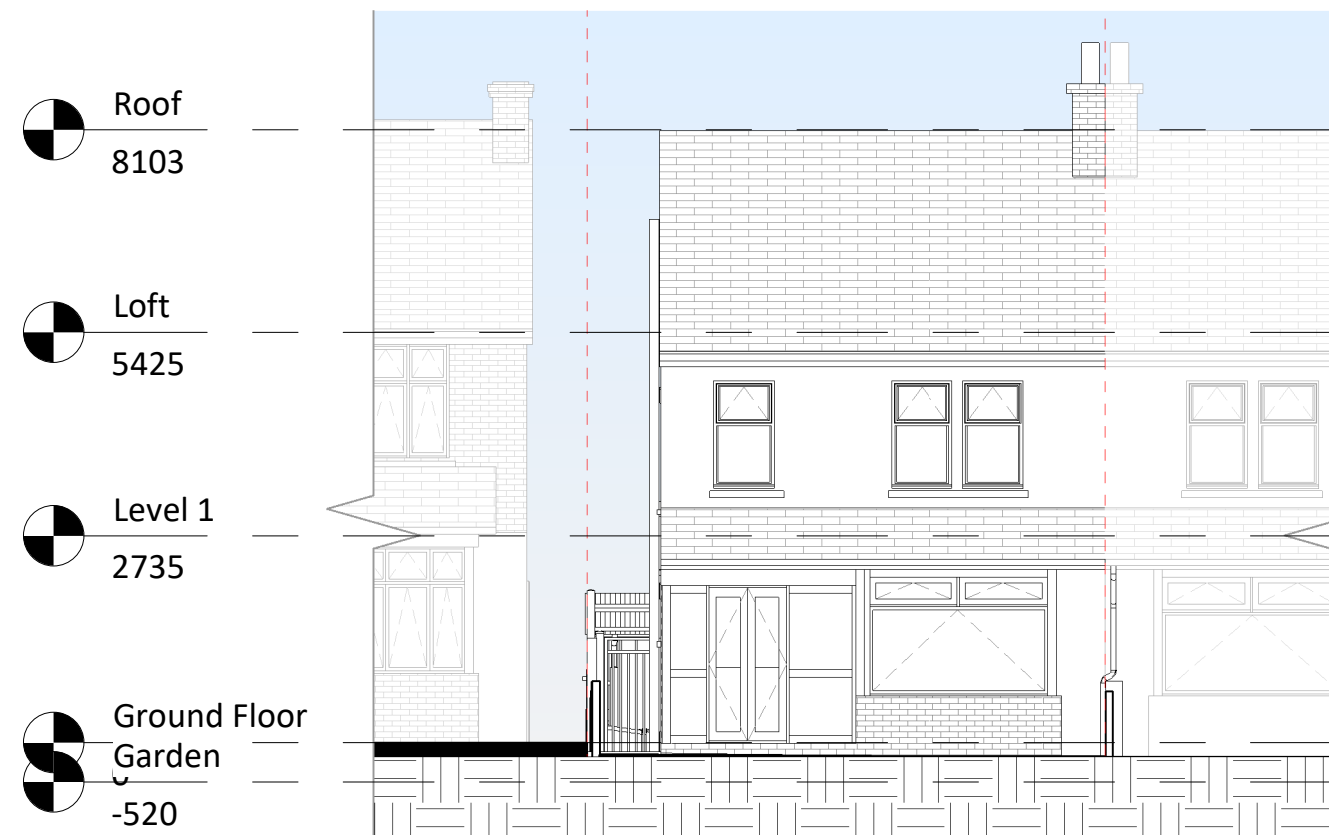
5 Existing Front Elevation 1 : 100
