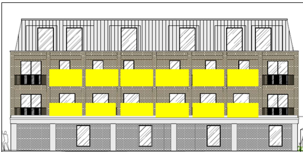
Fig. 1: Position of the 3 sided 1.5m high glass or equivalent solid balcony screens – drawing 1586-06
