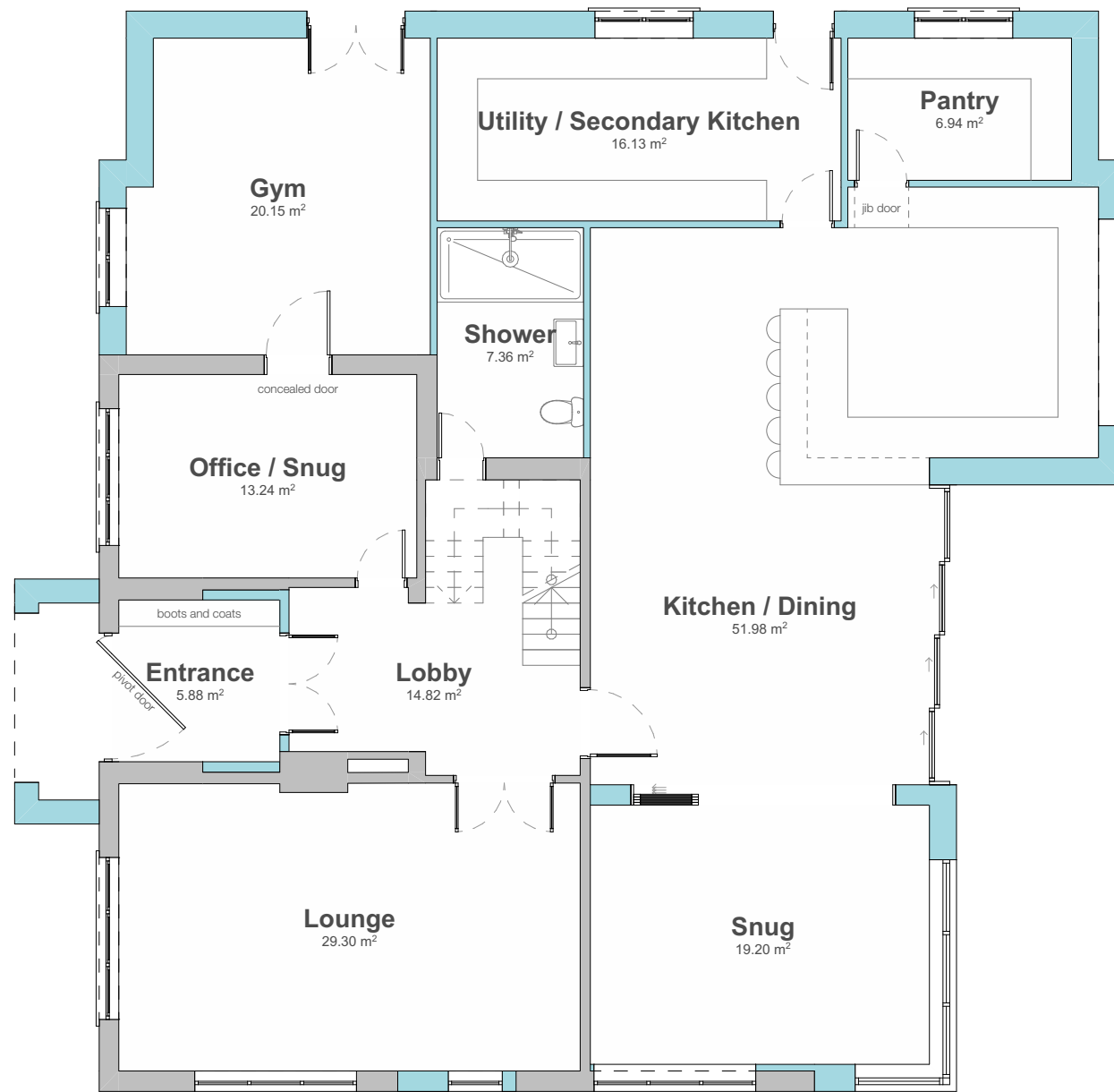
Proposed Ground Floor Plan Scale 1:100 @ A3
