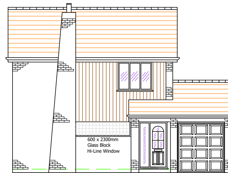
Existing Front (North) Elevation 1:100
