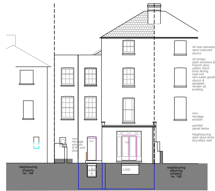
As Built West Facing Elevation @ scale 1:200
