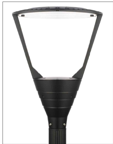
IP66 LED Premium Post Top Lantern 4000-4500k colour temp. 60W & 6900 lumens. Fitted with dawn till dusk photo cell. Set on min. 3m high post
