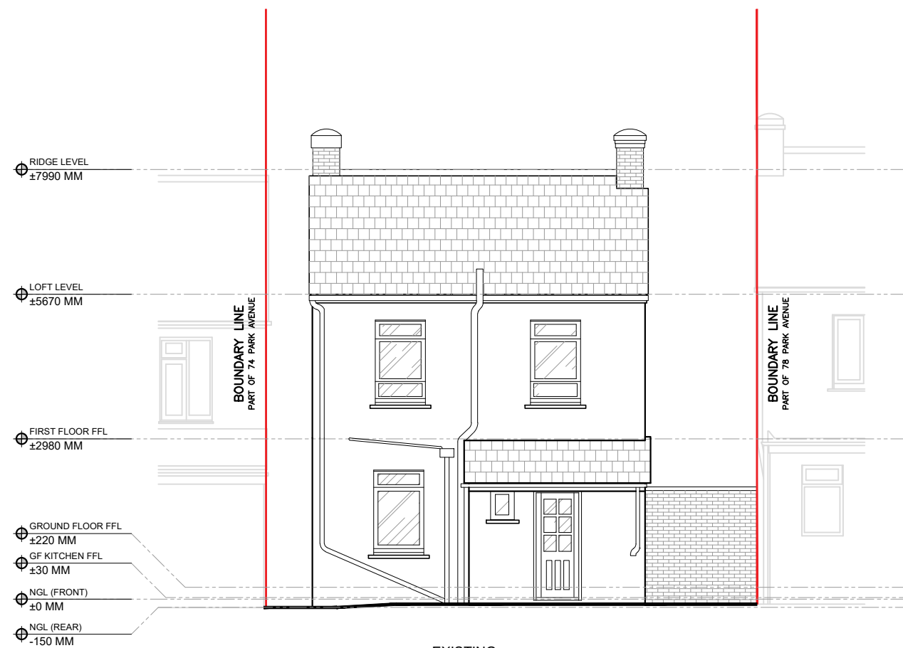
1 A07 EXISTING REAR ELEVATION SCALE 1:100
