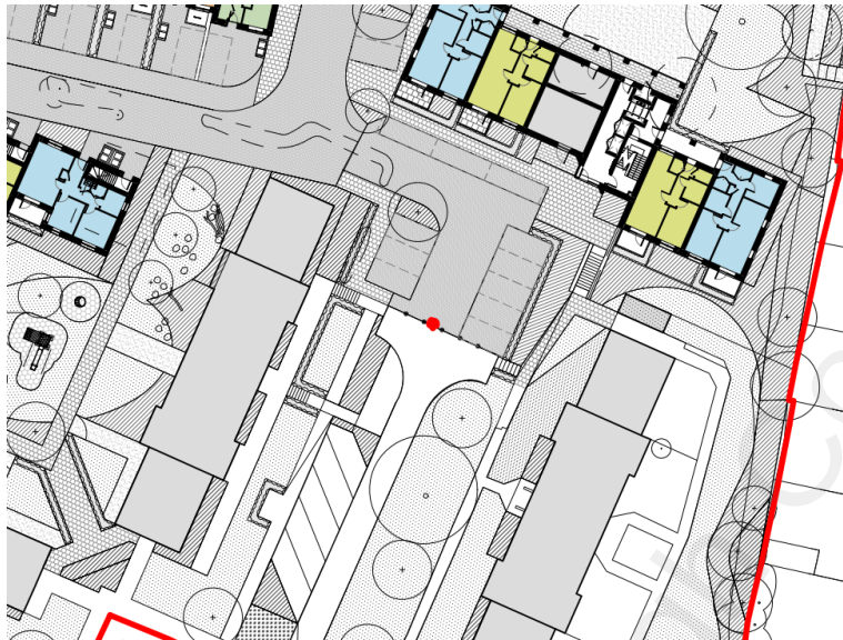
Figure 3.2 – Approximate Location of Collapsible Bollard
