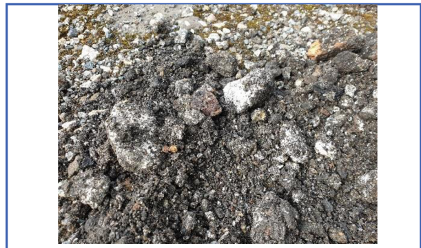
BH201 arising to 2.7m bgl
