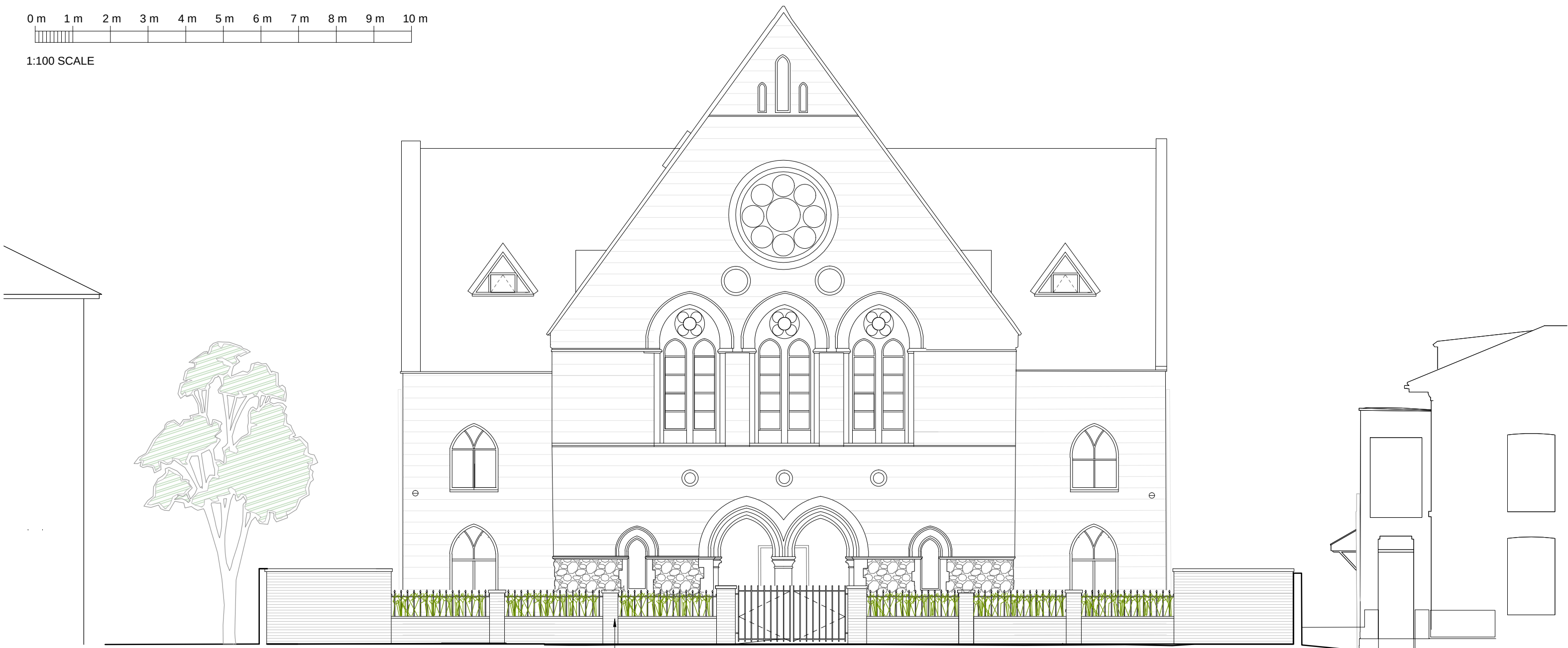
Yellow stock brick boundary wall with stone coping, black metal railings and entrance gates.
