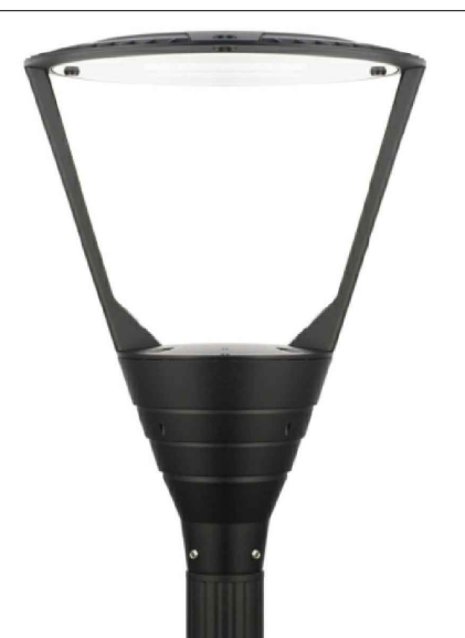
IP66 LED Premium Post Top Lantern 4000-4500k colour temp. 60W & 6900 lumens. Fitted with dawn till dusk photo cell. Set on min. 3m high post
