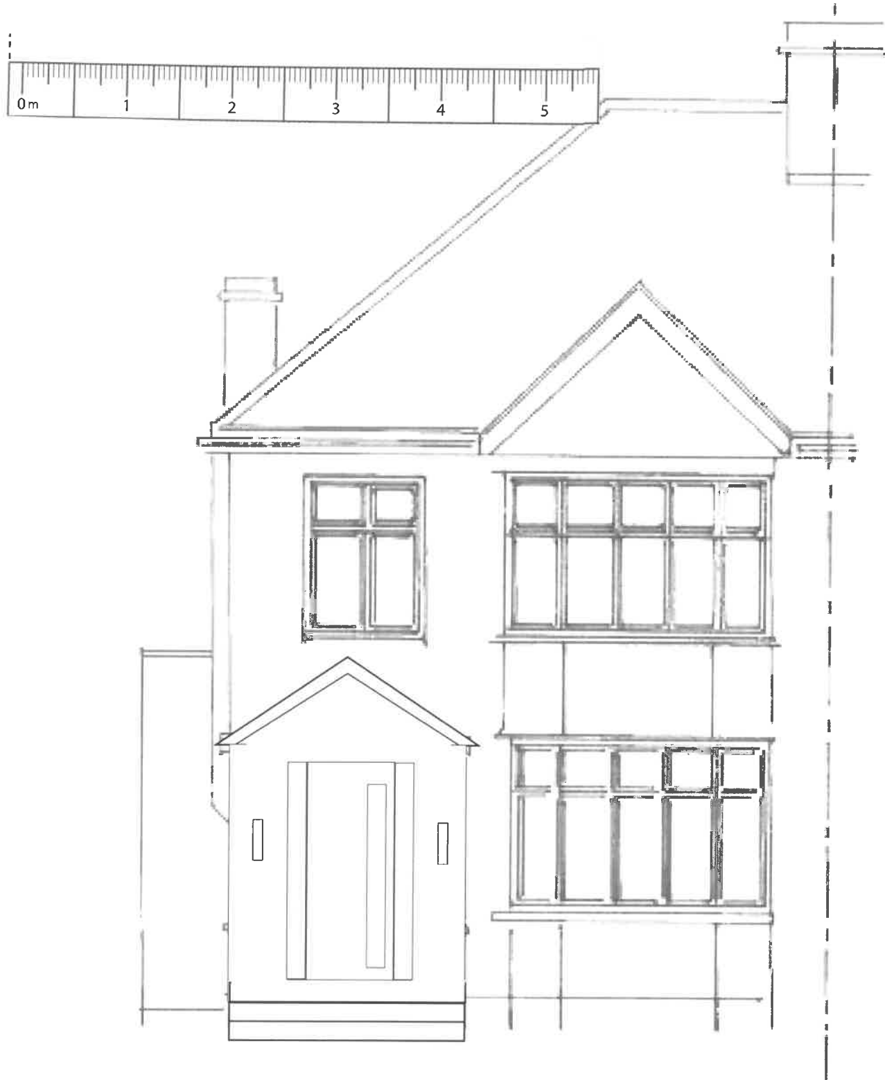
Front Elevation with addition Of new porch
