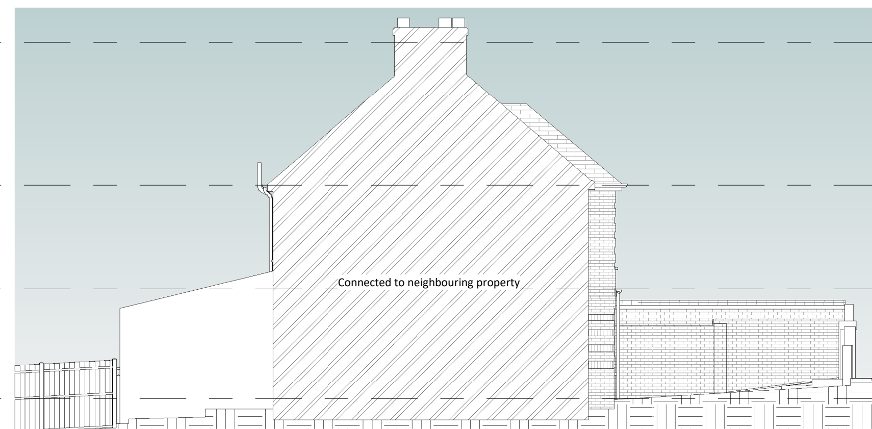
8 Existing West Elevation 1 : 100
