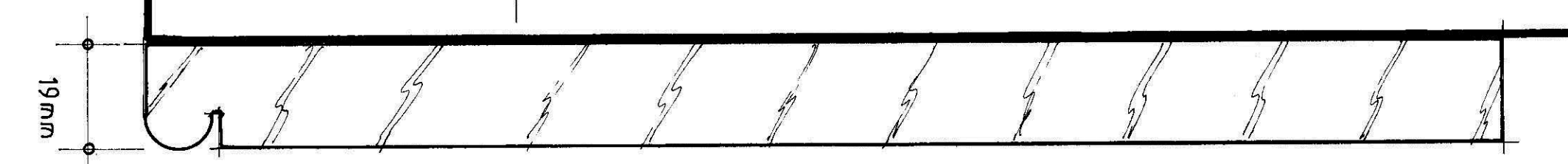
Full size section B-B JAMBS 19 x 24mm (24 INCLUDES 13mm BEAD). 2x 9mm DEEP (INCLUDING CHAMFERS) HORIZONTAL LEDGES.
