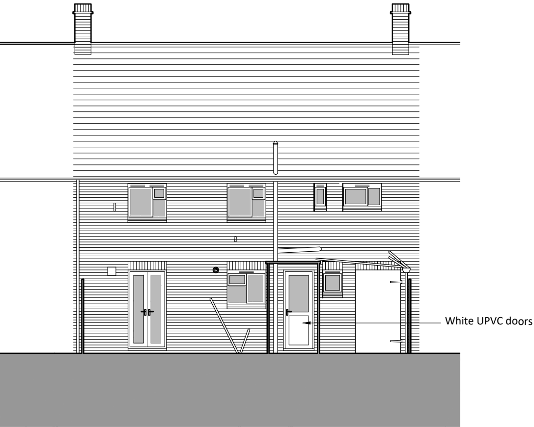
Existing Rear (South-West) Elevation 1100
