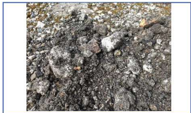
BH201 arising to 2.7m bgl
