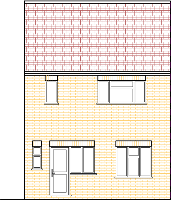
Existing Rear Elevation
