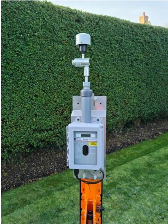
Fig. 8 Air Quality (Dust) Monitoring Equipment
