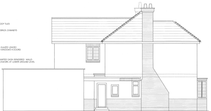
EXISTING SIDE ELEVATION
