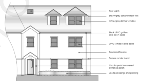
Proposed Rear Elevation 2 (North-West Facing) SCALE 1:100
