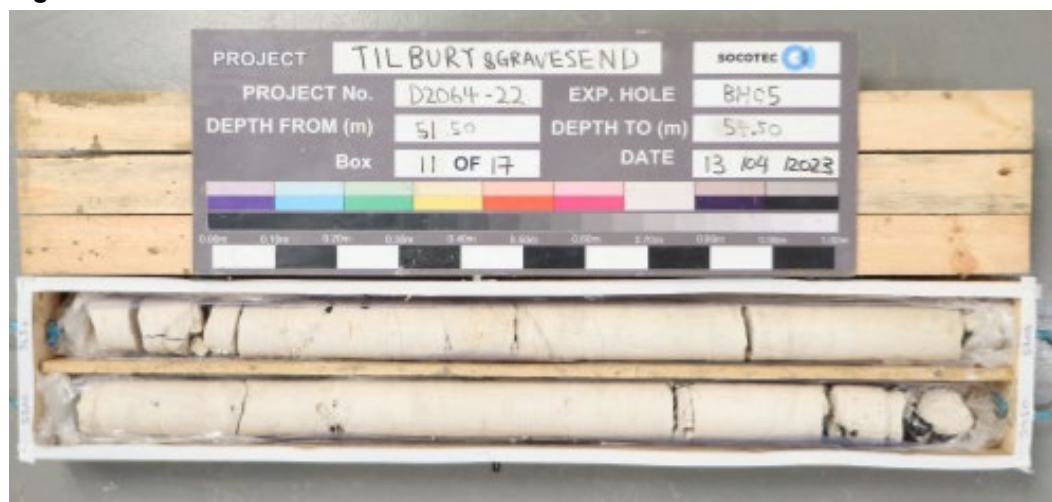
Figure 6. BH05 51.50m to 54.50m core CIRIA Grade A1 Seaford Chalk Formation
