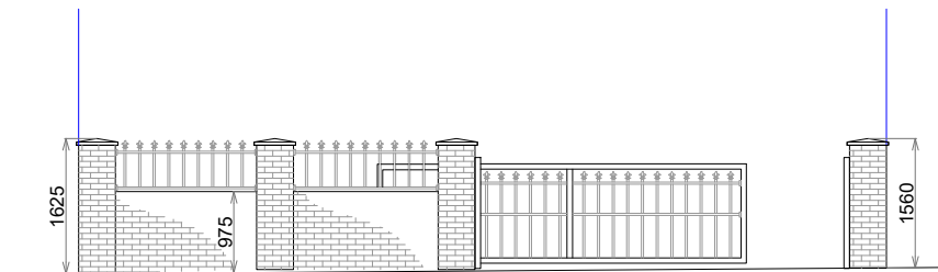
EXISTING FRONT ELEVATION
