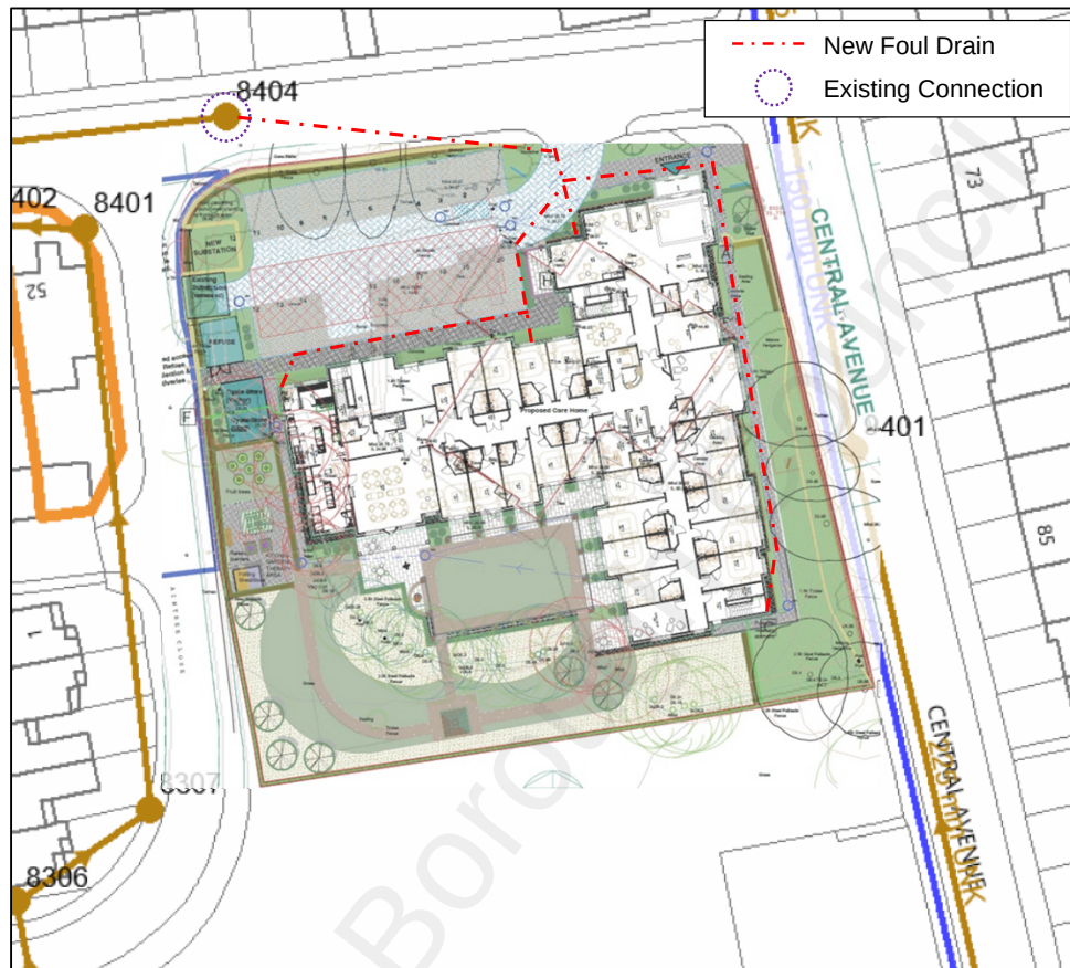
Figure 6.1 – Indicative foul drainage layout plan.
