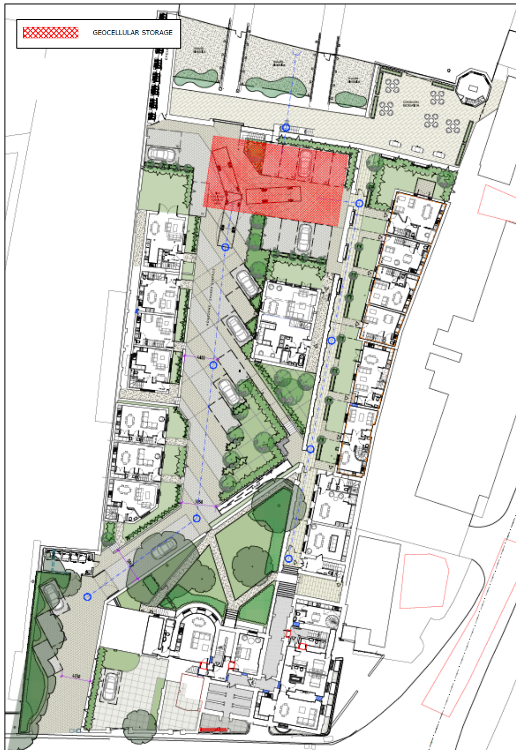
Figure 8.1 - Indicative drainage layout plan showing the proposed location of SuDS.
