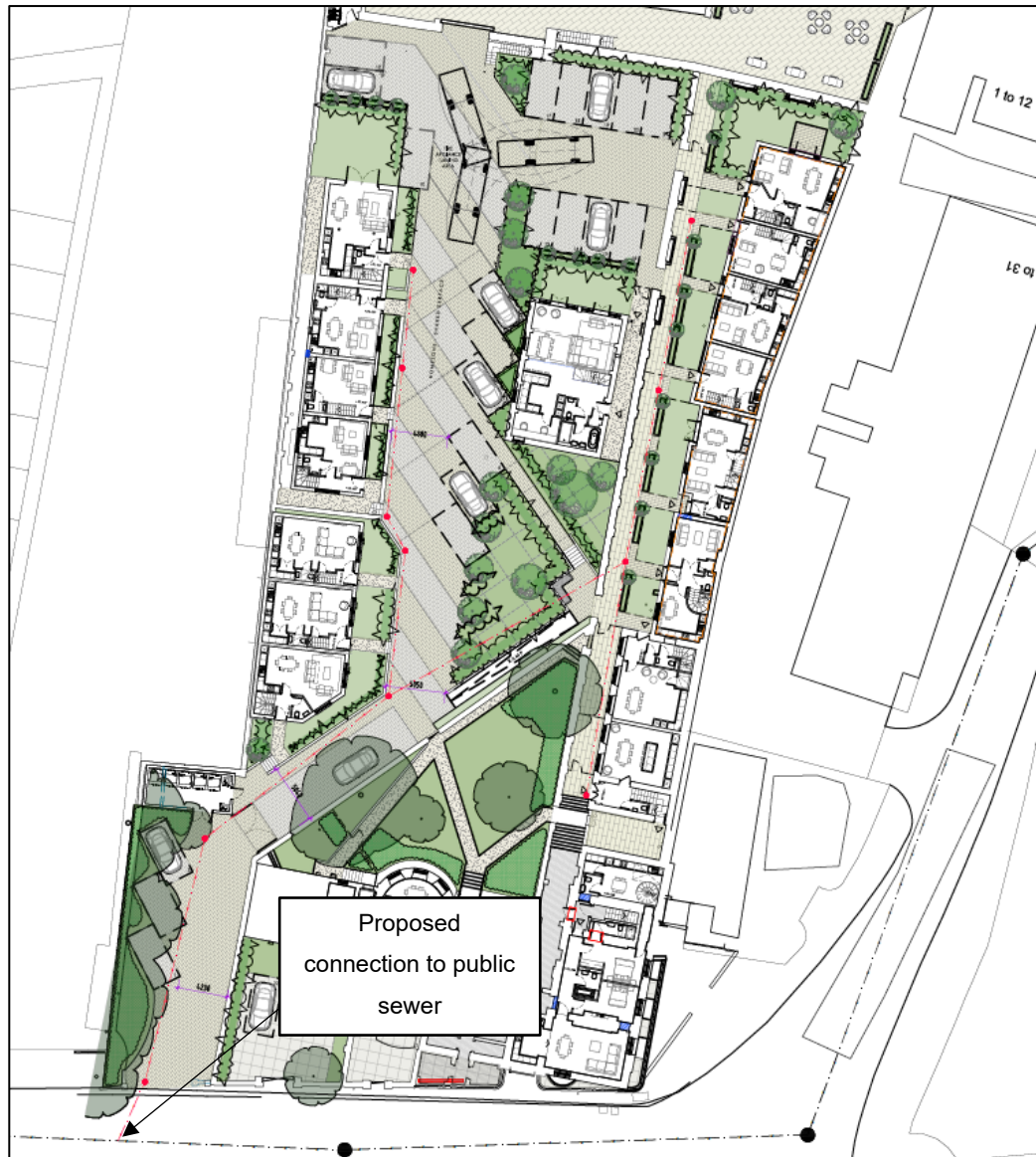
Figure 9.1 – Proposed connection to foul sewer network.
