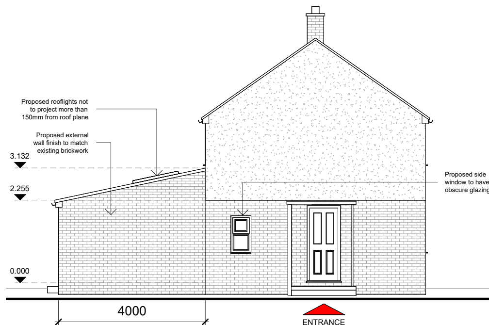
4 Side Elevation (North) 1 : 100
