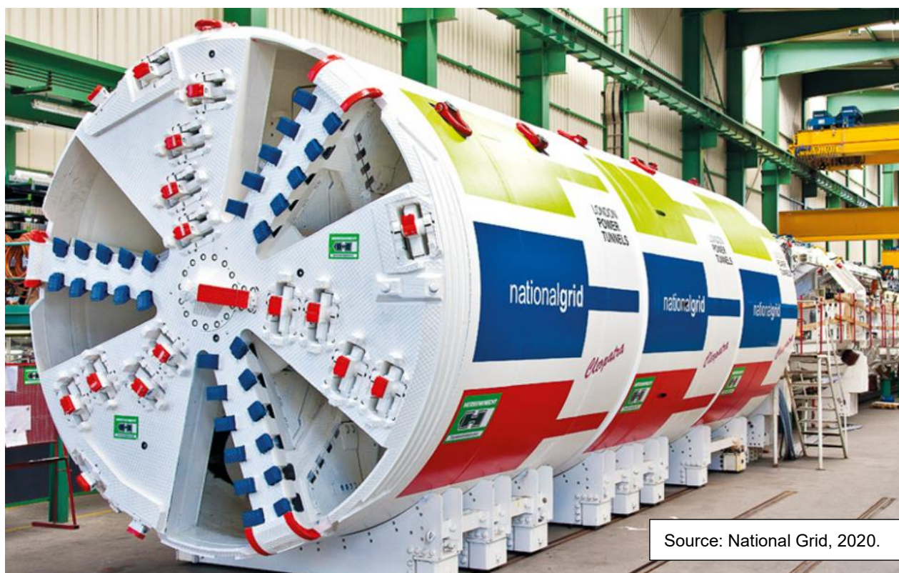
Figure 3-7: Example Tunnel Boring Machine
