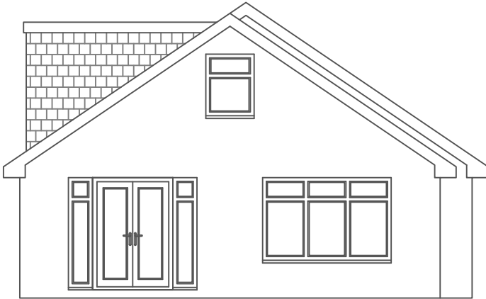
Proposed Rear Elevation Scale 1:100
