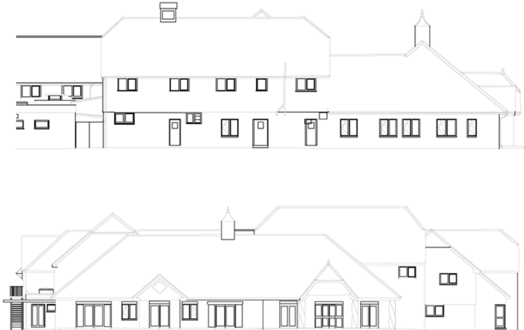
Fig 004 – external fenestration alterations to south and east elevations
