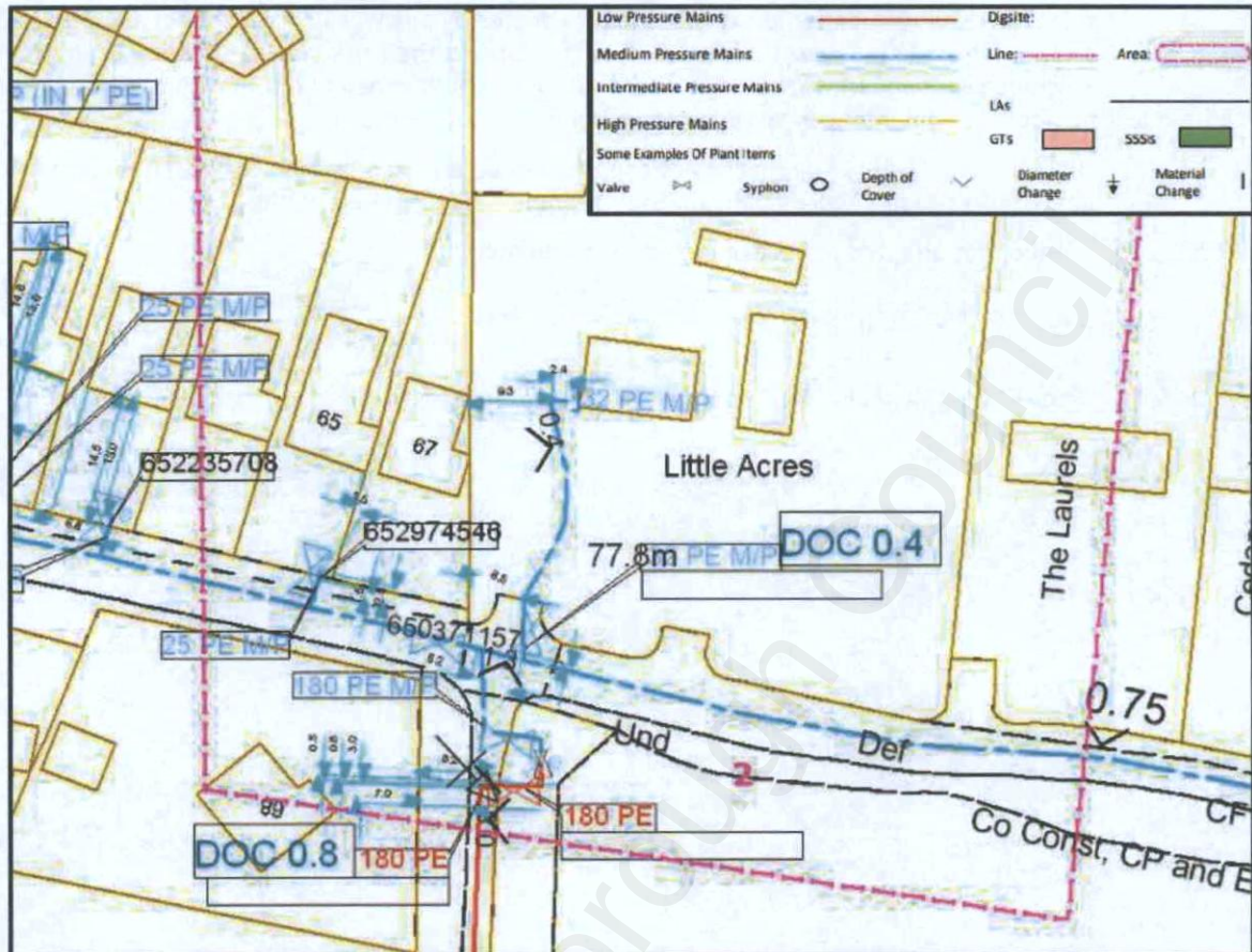
Figure 4 - Extract showing gas pipelines in relation to the site as per SGN Map
