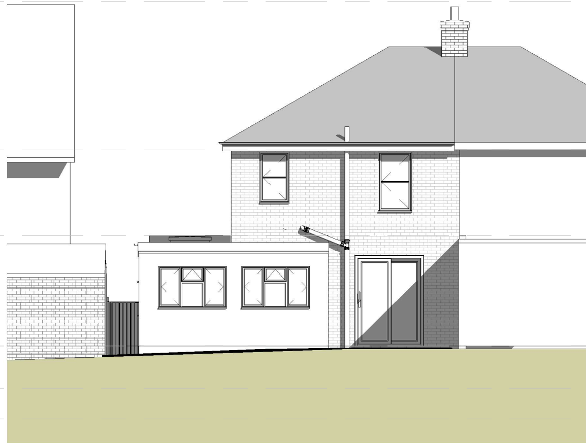
② 02 - Rear Elevation Proposed 1 : 100
