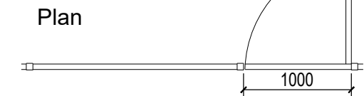
Plan Boundary Type B-C, C-D, D-E 1800mm high loop-top black metal fence & secure access gates. Scale 1:50
