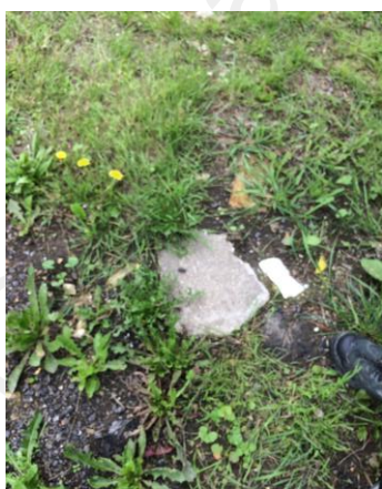
Plate 5- Asbestos cladding found on the surface around the site.
