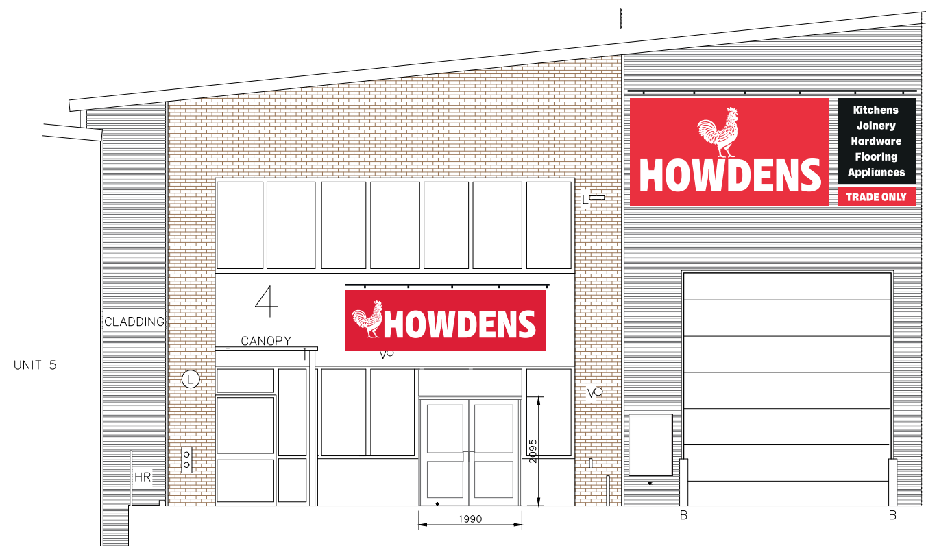
ILLUMINATED SIGN 3 - 4000mm x 1150mm x 80mm
