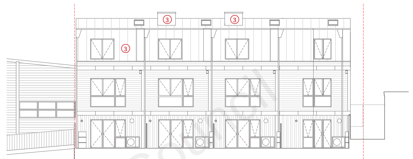
Application of metal cladding to East Elevation
