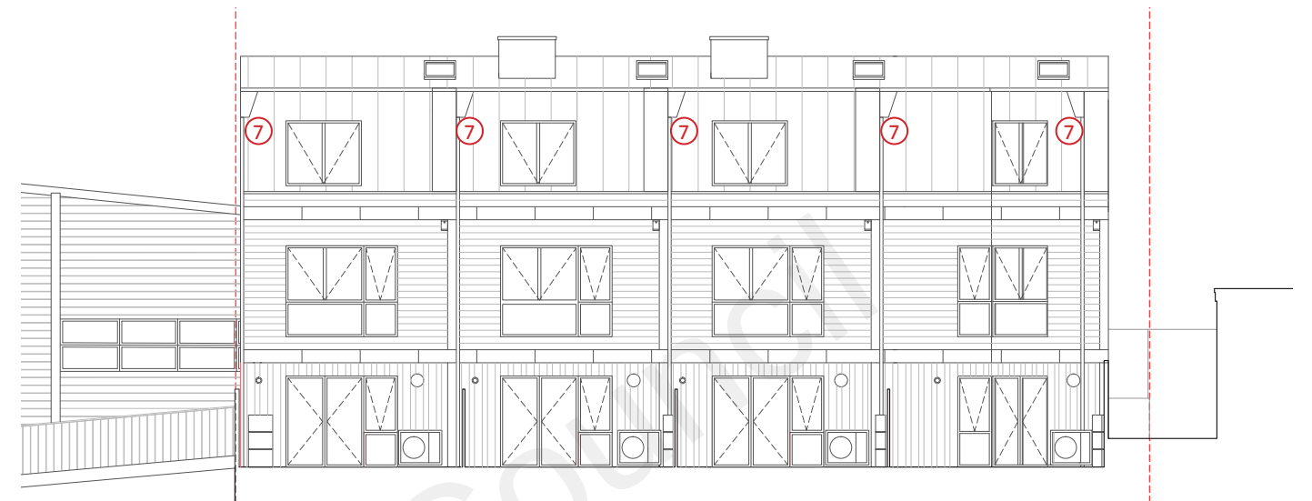
Application of rainwater goods to East Elevation
