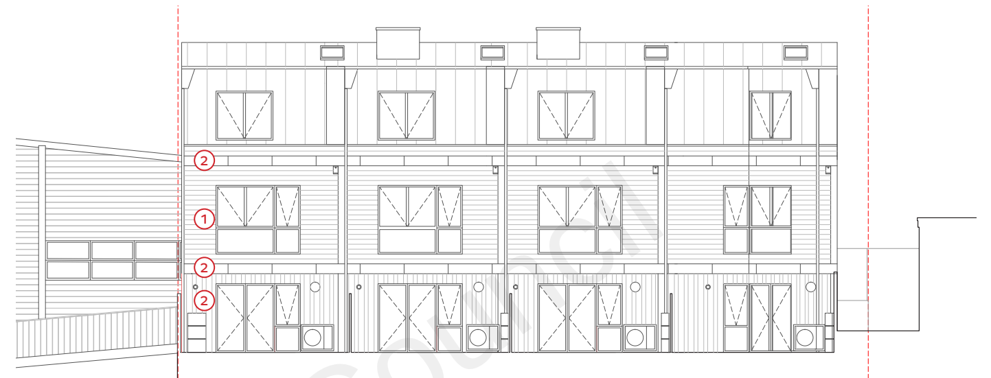
Application of fibre cement planks to East Elevation
