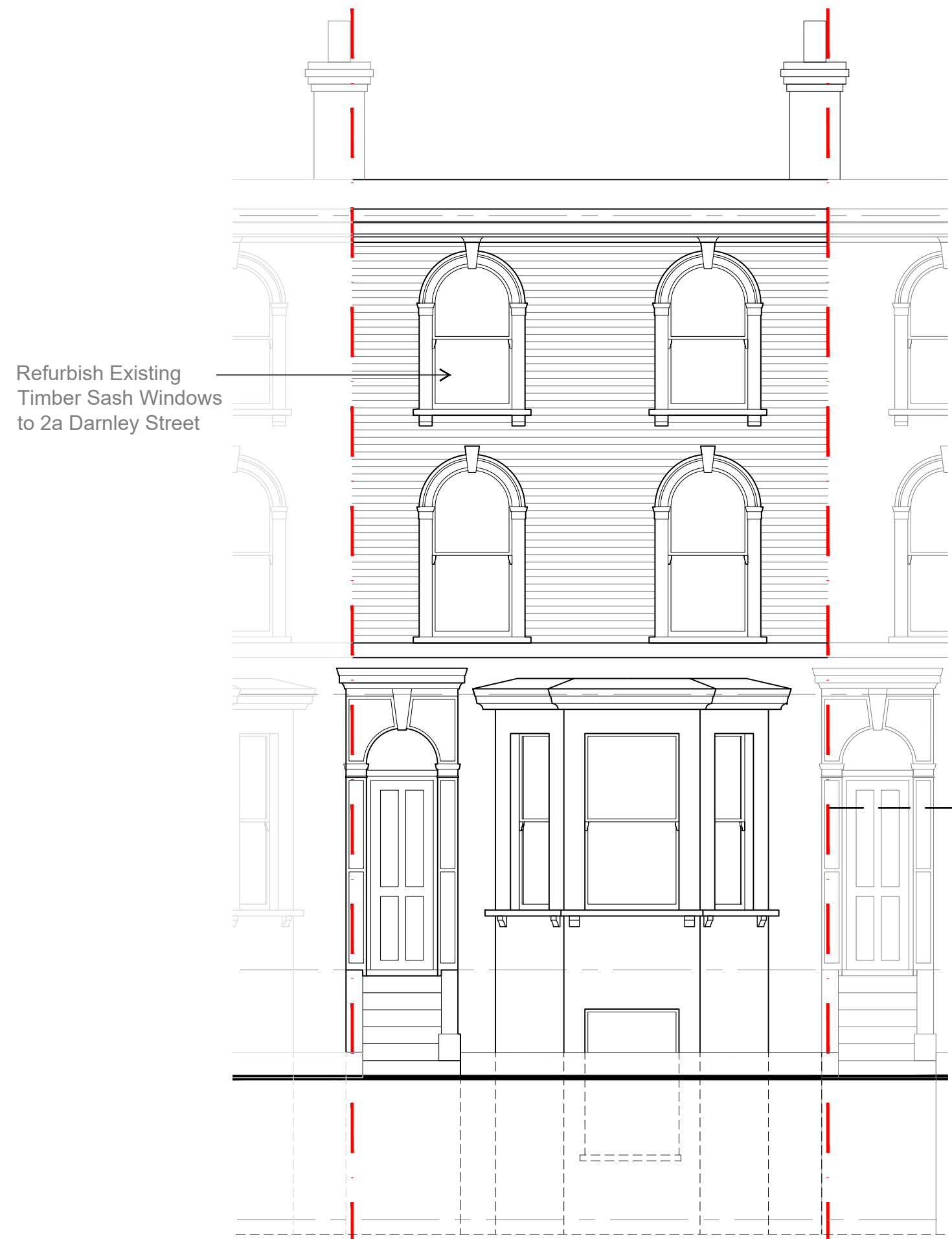
01 (01)700 North Elevation - As Existing Scale 1:50
