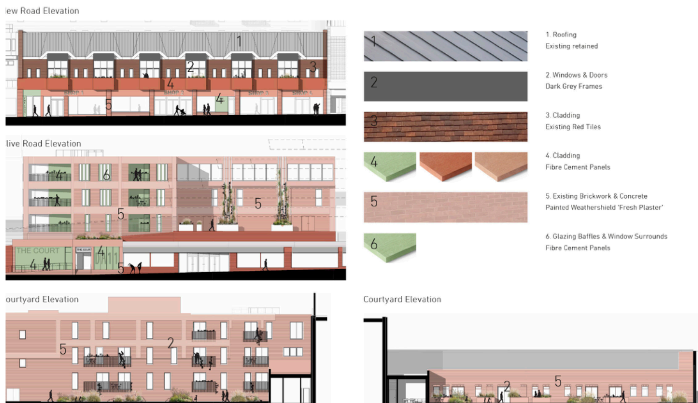
Figure 11: Transformation of facade
