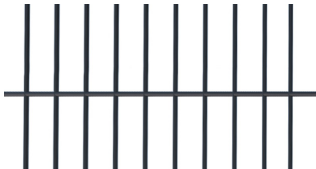
ZedPanel V-Mesh Black • 4mm Vertical Wire / 5mm Horizontal Wire/ 200mm x 50mm Aperture Size • Colour Coated Wire Black
