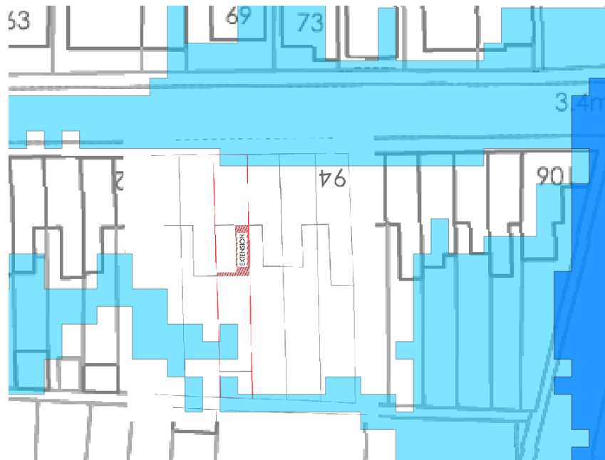
Figure 6: SW flood extent mapping. The extension is not shown to be at risk from SW flooding.
