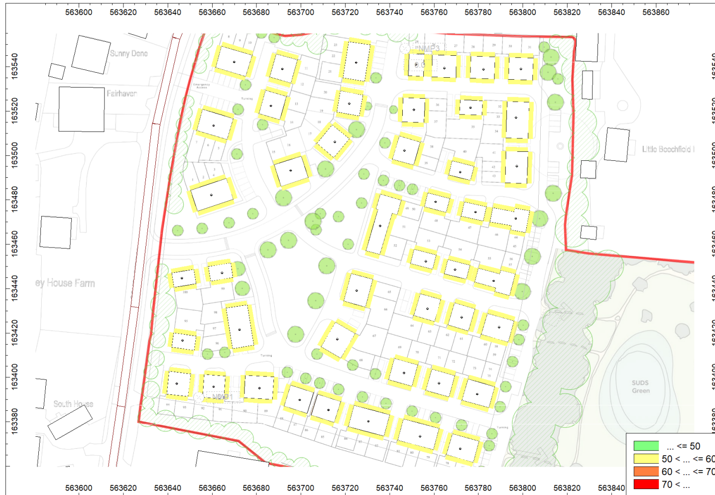
Figure D: Prediction of Road Noise Levels – Day L_{Aeq,16h}
