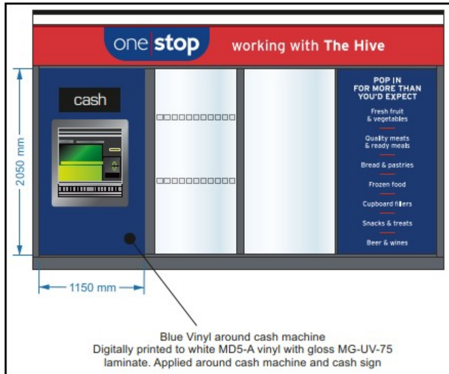
6) LHS False ACM Window Panels,
