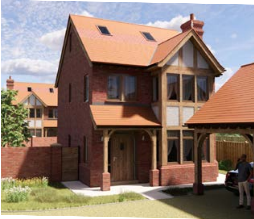
Facing bricks - Red multi Butterley Red Bank Coronet. Mortar colour to match brick. Oak timber posts
