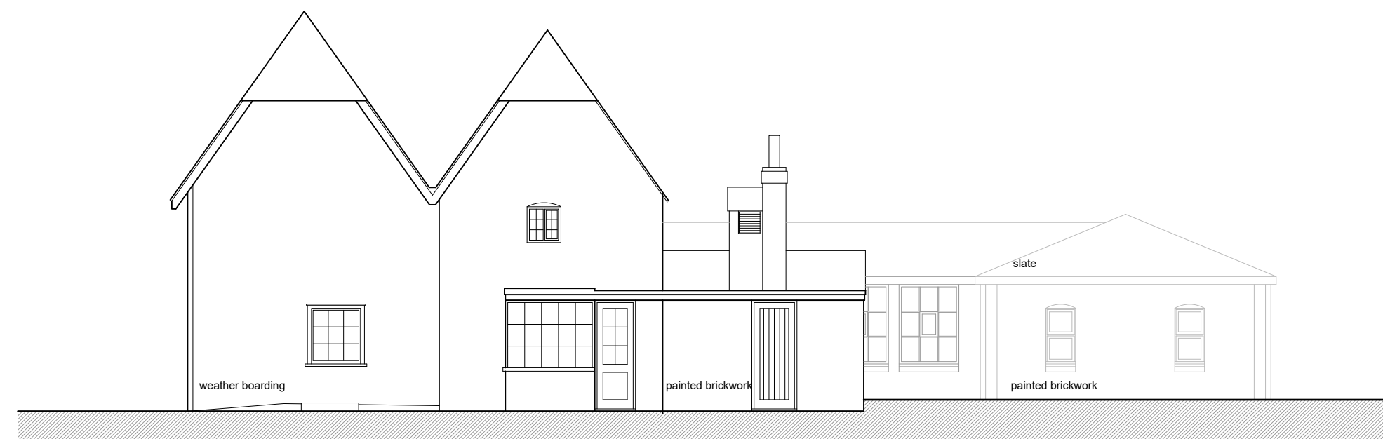
Side Elevation - North Existing scale 1:100 @ A1
