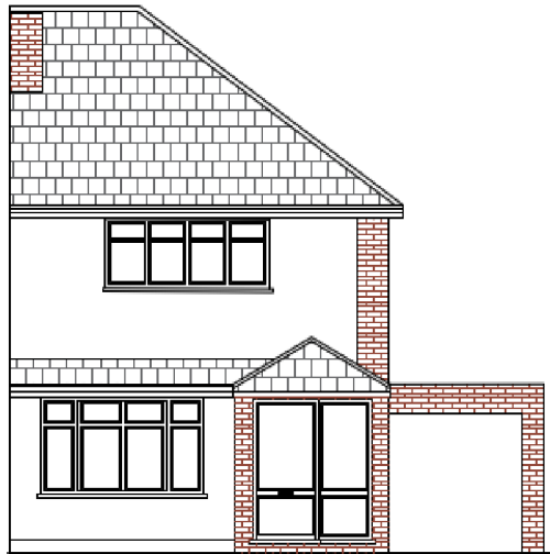
EXISTING FRONT ELEVATION 1:100
